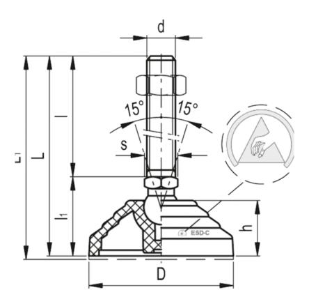
$$\begin{aligned} & \text{Max load} & = 14000 \\ & \text{s} & = 16 \\ & \text{Weight in (g)} = 290 \end{aligned}$$
